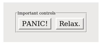
Here is an example of a LabelFrame widget containing two Button widgets. Note that the label "Important controls" interrupts the border. This widget illustrates the default GR00VE relief (see Section 5.6, "Relief styles" (p. 11)) and the default 'nw' label anchor, which positions the label at the left side of the top of the frame.
