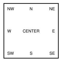
For example, if you create a small widget inside a large frame and use the anchor=SE option, the widget will be placed in the bottom right corner of the frame. If you used anchor=N instead, the widget would be centered along the top edge.
