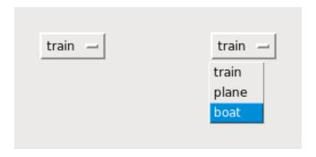
The illustrations above shows an <code>OptionMenu</code> in two states. The left-hand example shows the widget in its initial form. The right-hand example shows how it looks when the mouse has clicked on it and dragged down to the <code>"boat"</code> choice.
